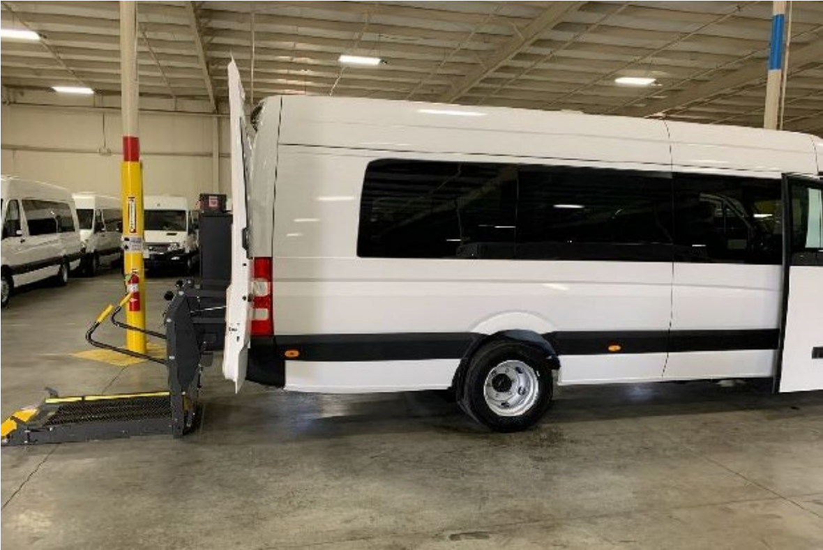
Wheelchair ramp getting ready to be installed in an EV Star
