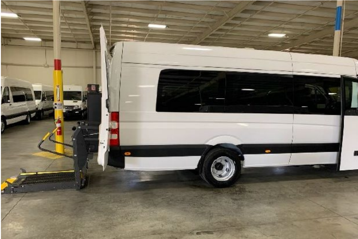
Above is a wheelchair ramp being installed in an EV Star.
